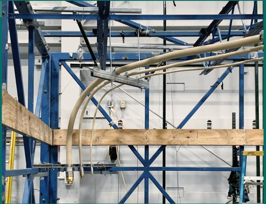
*MediTrac® CMT in seismic test rig.*
